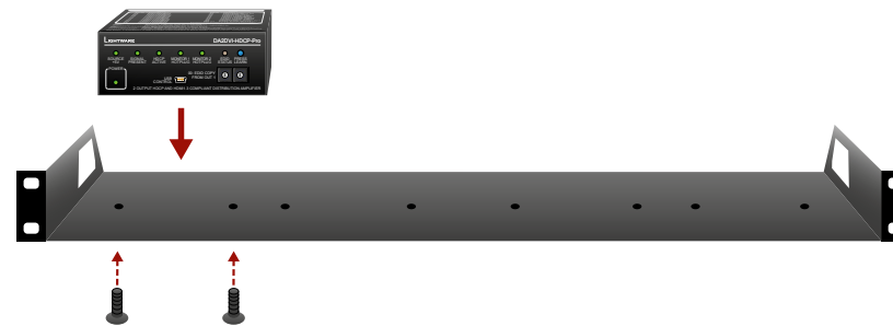
Mounting with 1U-high Rack Shelf
